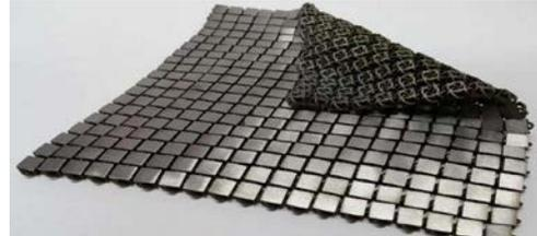
NASA has designed a woven metal fabric that combines fashion and engineering. Its main characteristics are reflectivity, passive heat management, foldability and tensile strength. It could have a wide variety of uses, in antennas, shielding spacecrafts from meteorites and for spacecraft insulation.
